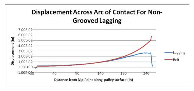
Figure 7 – Belt and Lagging displacement vs. Location along face of pulley.
