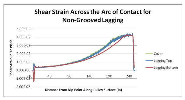
Figure 8 – Shear Strain vs. Location along face of pulley
