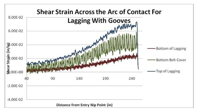
Figure 10 – Shear Strain vs. location along the arc of contact for different components within the lagging model for Grooved Lagging.
