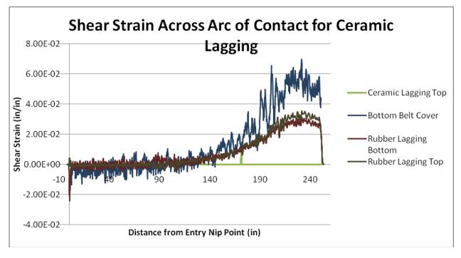
Figure 11 – Shear Strain vs. location along the arc of contact for different components within the lagging model for Ceramic Lagging.
