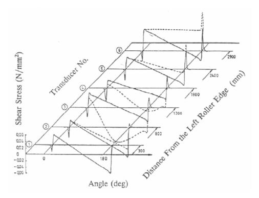
Figure 9 - Figure showing the result slippage has on shear stress along the face of the pulley (transducers 3 and 4).
