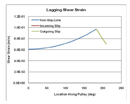
Figure 5 – Shear Strain vs. Location along face of pulley.
