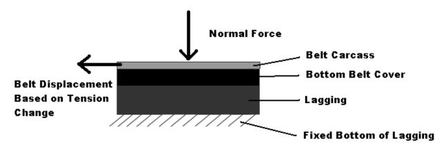
Figure 6 – Diagram showing general FEA model geometry
